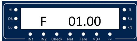
Set the spill weight. In this example, the filling target is 5.00kg, the spill setpoint is 0.30kg. That means the fine feed output status will change from active to inactive while the filling weight over ( $5.00 - 0.30 = 4.70$ )kg.
