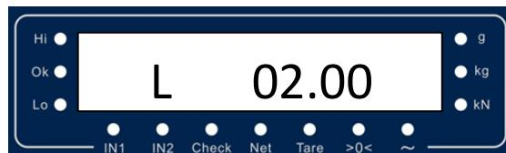
Set the refill sequence stop value. the terminal set the refill output inactive if the refilling weight be over this value.
