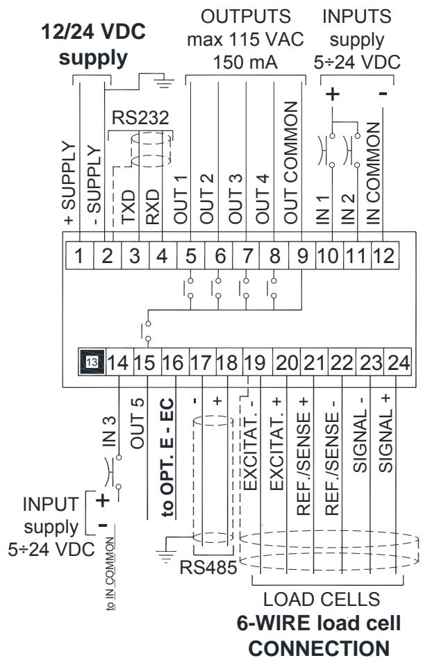
**5 outputs:** controlled by setpoint values or by remote device via protocol.
